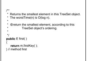
The TreeSet class has the same methods as the BinarySearchTree class, but is faster, at least in the worst case. For add, remove, and contains, worstTime(n) is logarithmic in n, versus linear in n for the BinarySearchTree class.
